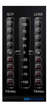
In addition to, the information display panel of the DNYK propulsion control system can observe the current position of the currently controlled lever and the driven lever to minimize the misoperation.
