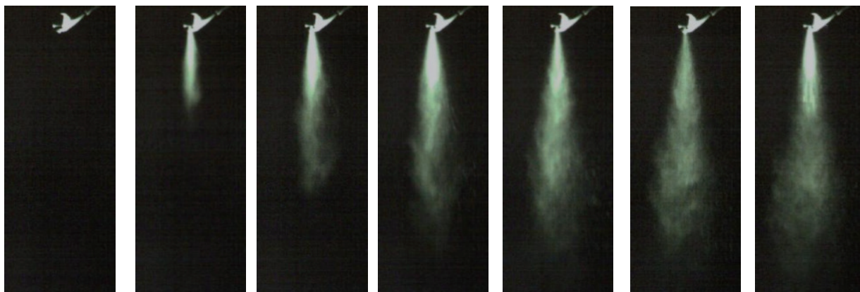
喷雾发展过程高速摄影图片 Mist development process high-speed photography pictures
